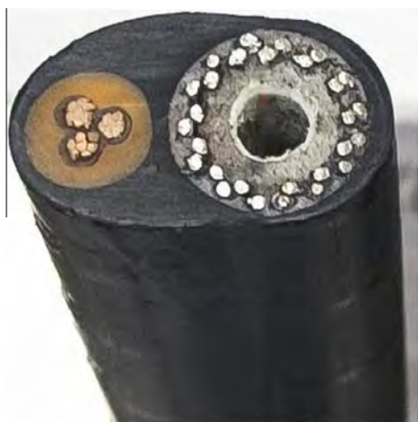
Fig. 8. Possible design of a cable for sonochemical treatment of wells with high-viscosity oil on a permanent basis.
